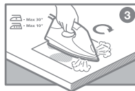
Place the hot iron on the surface that needs repairing. Do not leave the iron on the surface for more than 10 seconds at a time.
