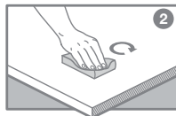
Rub the magic sponge on the area where the micro-scratches can be seen. The sponge can be used dry or slightly damp.
